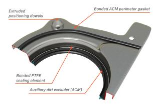
For rear crank seal applications, the oil seal housing and gasket are often now combined into a single unit known as an integrated oil seal which also provides a better level of overall sealing ability. The design of these integrated oil seals means that replacement of the individual sealing elements is not feasible and the unit will need to be replaced as a complete item.
